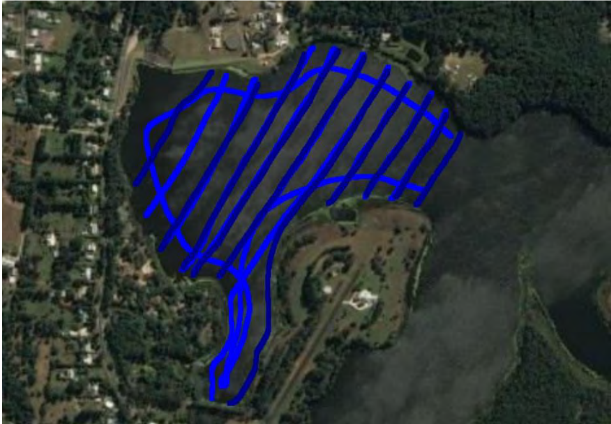
Figure 4. Typical survey transect pattern used in each zone recorded in the internal gps unit in the head unit of the DT-X.
