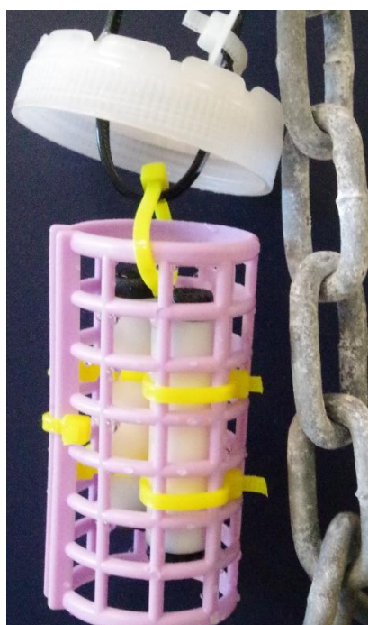
Figure 3. Microporous Polyethylene Tube (MPT) passive samplers for monitoring of PFAS in mesh enclosure
