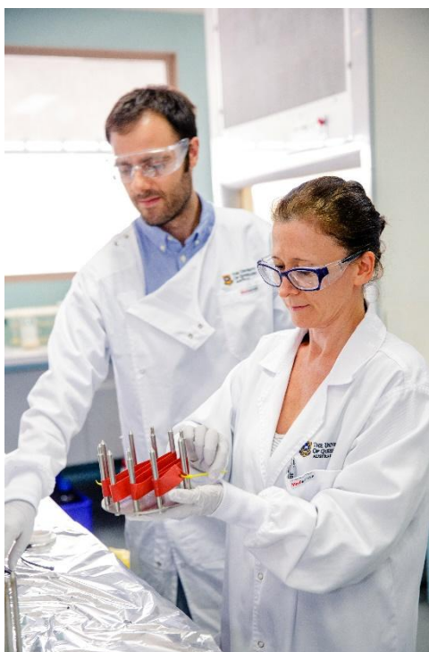
Figure 2. Preparation of a PDMS passive sampler in a stainless steel cage.
