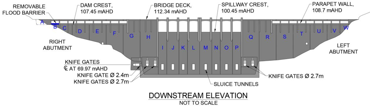
Figure 4.6.3 Somerset Dam typical cross-section pre-Early Works arrangement
