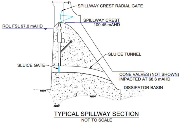
Figure 4.6.4 Somerset Dam typical cross-section post-Early Works arrangement
