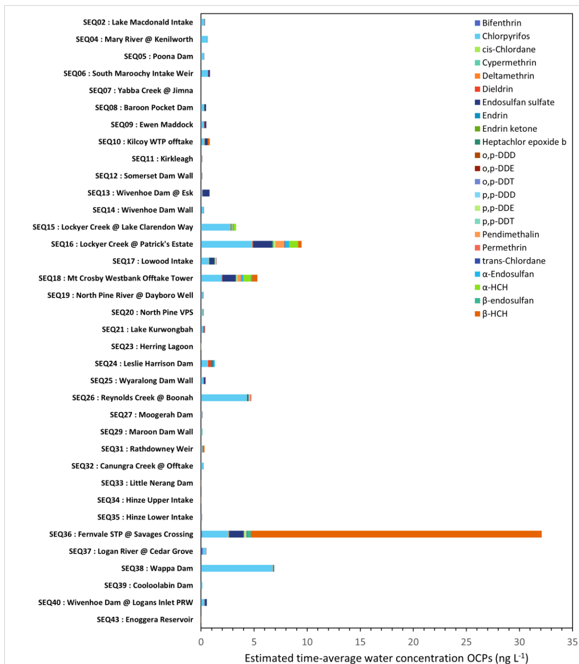
Figure 5. Total estimated water concentrations ( \text{ng L}^{-1} ) of 23 \Sigma OCPs (excluding Dacthal) at each site derived from PDMS passive samplers.
