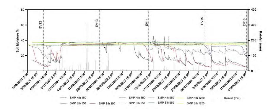
**Figure 6.** Soil moisture content (%) for the period covering four monitoring events from August 2021 to late September 2023 for both the Southern and Northern SMP's relative to floristic monitoring events. Significant data gaps are evident at the Northern SMP. The 350mm sensor at the Northern SMP has been omitted from this graph due to sensor malfunction.
