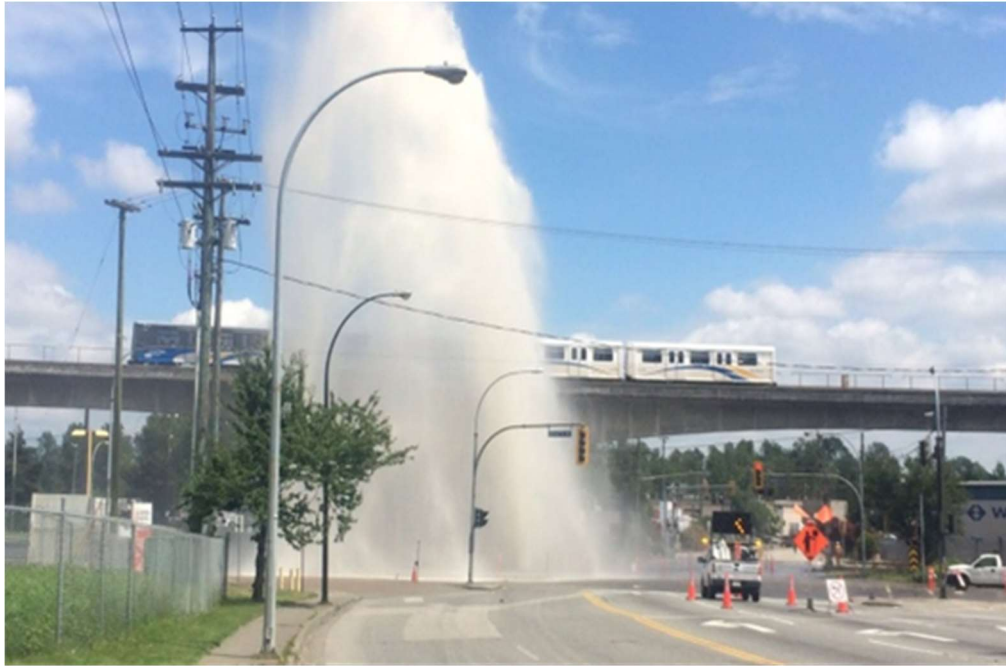
Figure 2-1: Due to the very high pressure at which Trunk water Mains operate; a break has the potential to release dangerous water jets.
