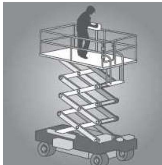
Figure 4: A scissor-lift elevated work platform.
