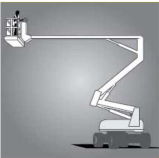
Figure 3: A boom-type elevated work platform. The safety harness and lanyard assembly are not shown for purposes of clarity. The lanyard should be as short as possible and should be attached directly to the designated anchor point on the elevated work platform, not to the handrail.
