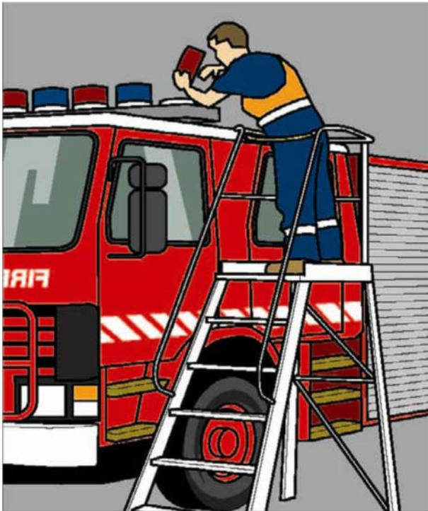
Figure 5: A platform ladder with a safety chain provides a stable work platform that allows the use of both hands to perform a work activity.
