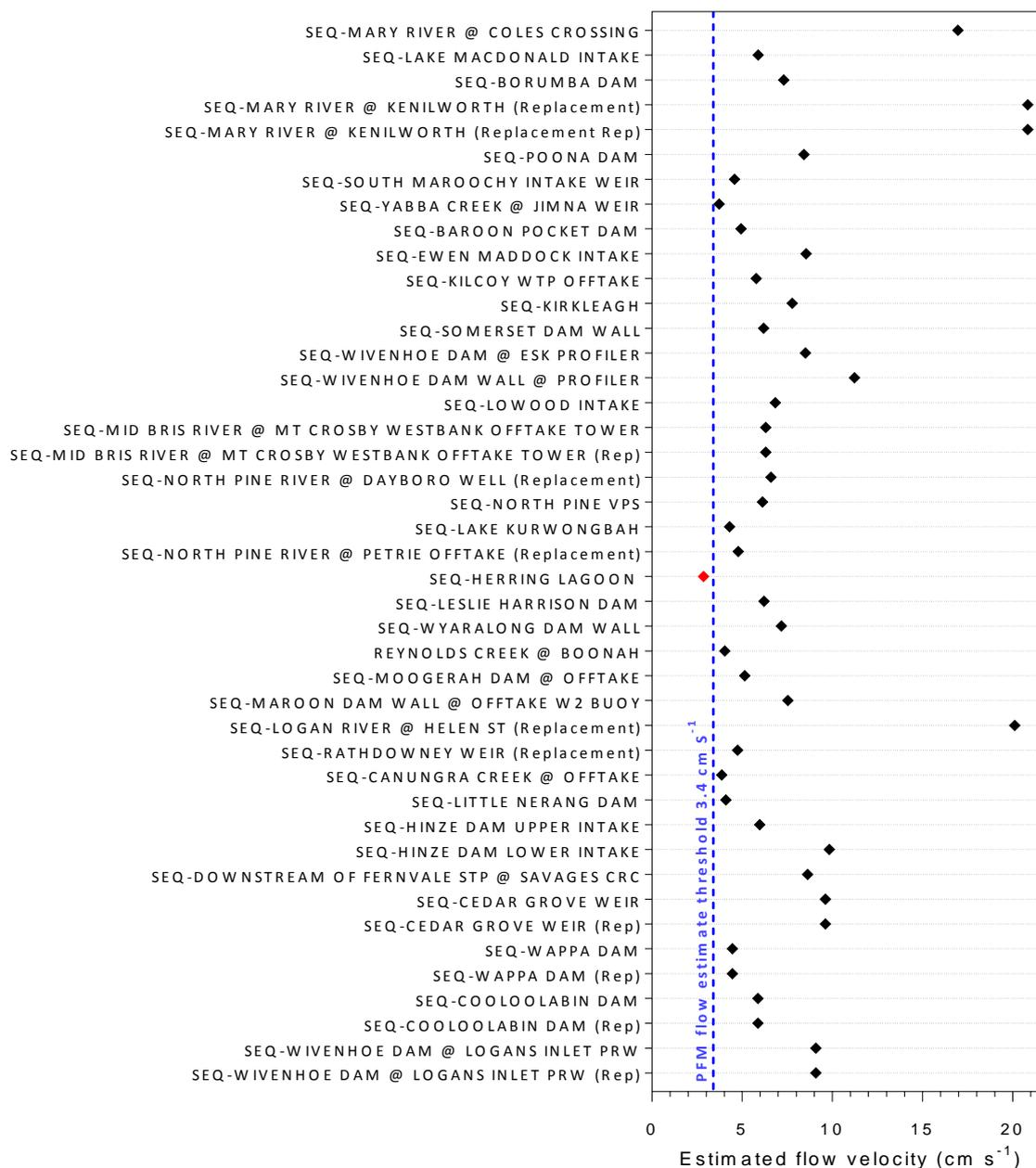
Figure 2. Passive flow monitor (PFM) based average water flow rate estimations at the deployment sites ( $n=37$ ). A minimum flow velocity of  $3.4 \text{ cm s}^{-1}$  is required in order to assess flow velocity using Passive Flow Monitors (PFMs). SEQ-HERRING LAGOON was the only site during this campaign to fall below the minimum flow velocity.
