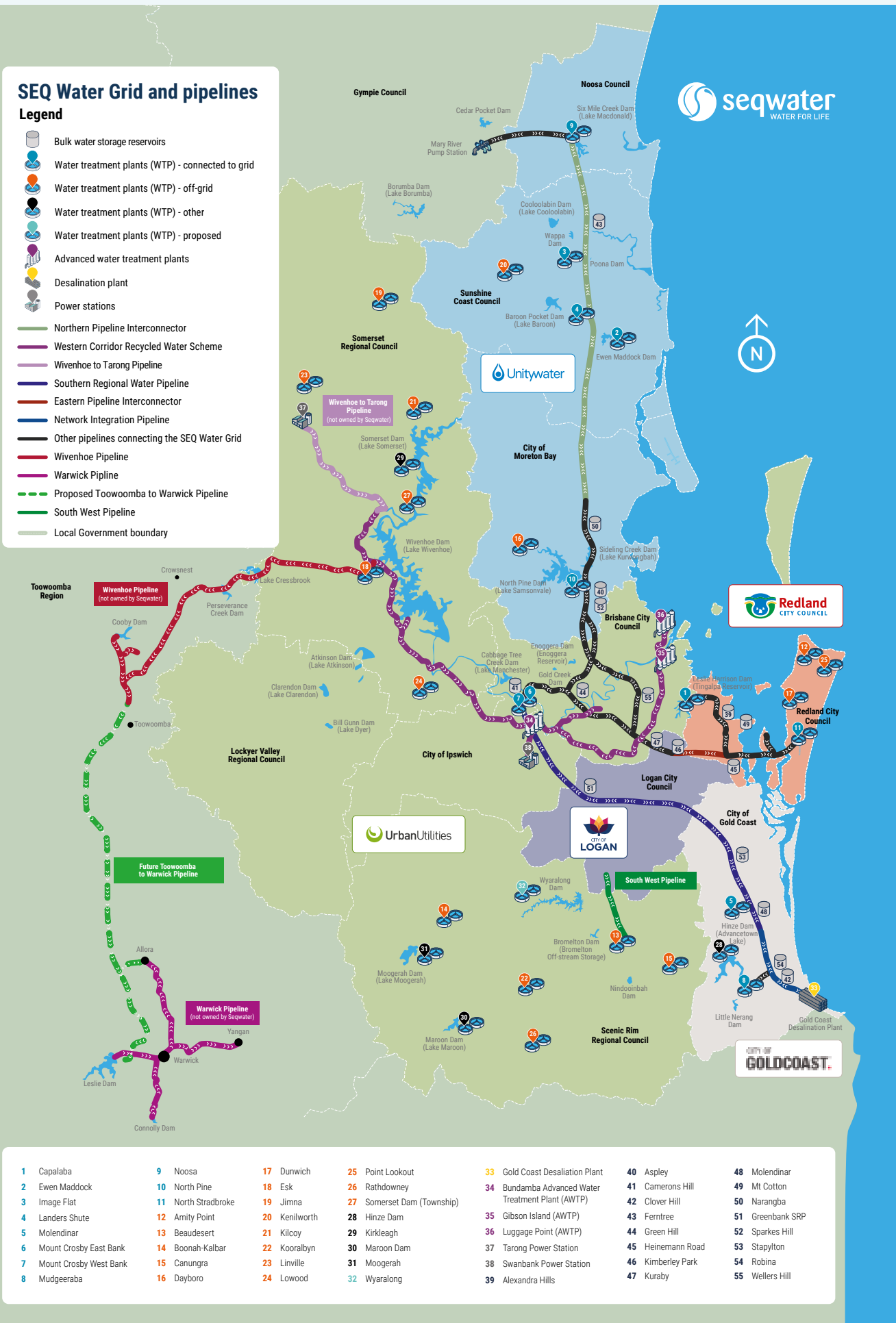
Figure 1: SEQ's Water Grid Supply Network
