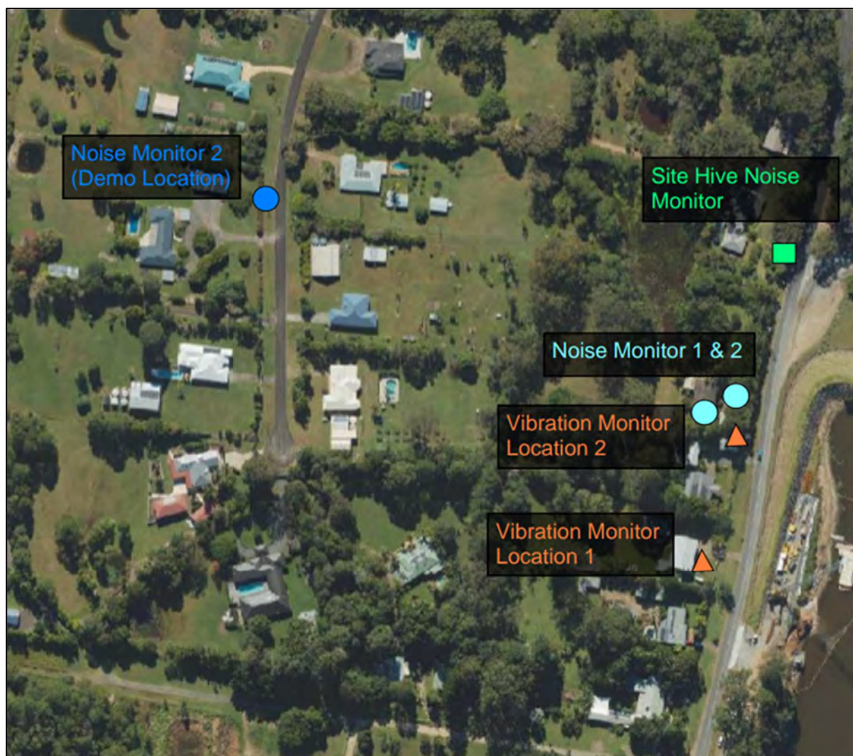
Figure 13: Noise and Vibration Monitoring Locations
