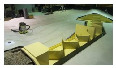
The hydraulic performance of the dam is assessed on the amount of water it can pass (release) through the spillway and the amount of energy dissipation the concrete area (basin) downstream can provide. A similar physical model dam was built to assess the hydraulic performance of the Hinze Dam spillway, which was upgraded in 2011.
