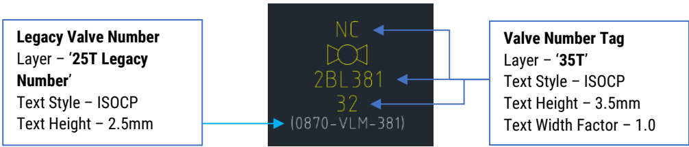
Figure 15 - Format & placement of valve tag text
