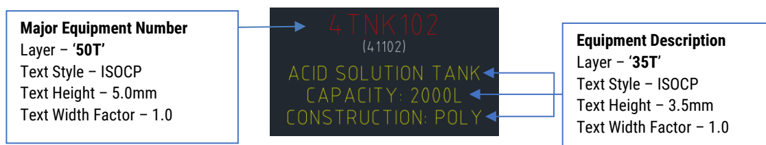
Figure 25 - Typical major equipment tag layout and format
