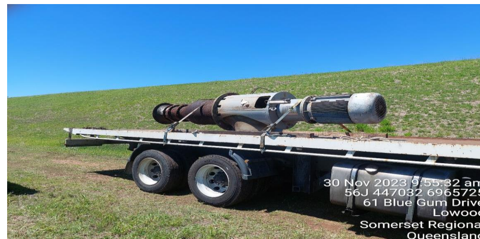
Figure 3: Pump 1 removed for refurbishment from Atkinson Dam and reinstalled April 2024.
