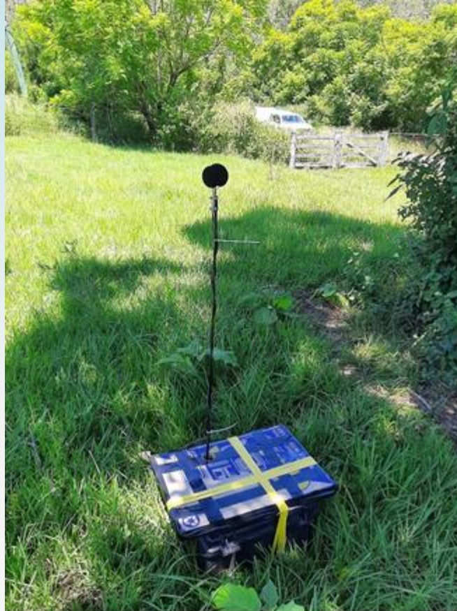
Baseline noise monitoring
