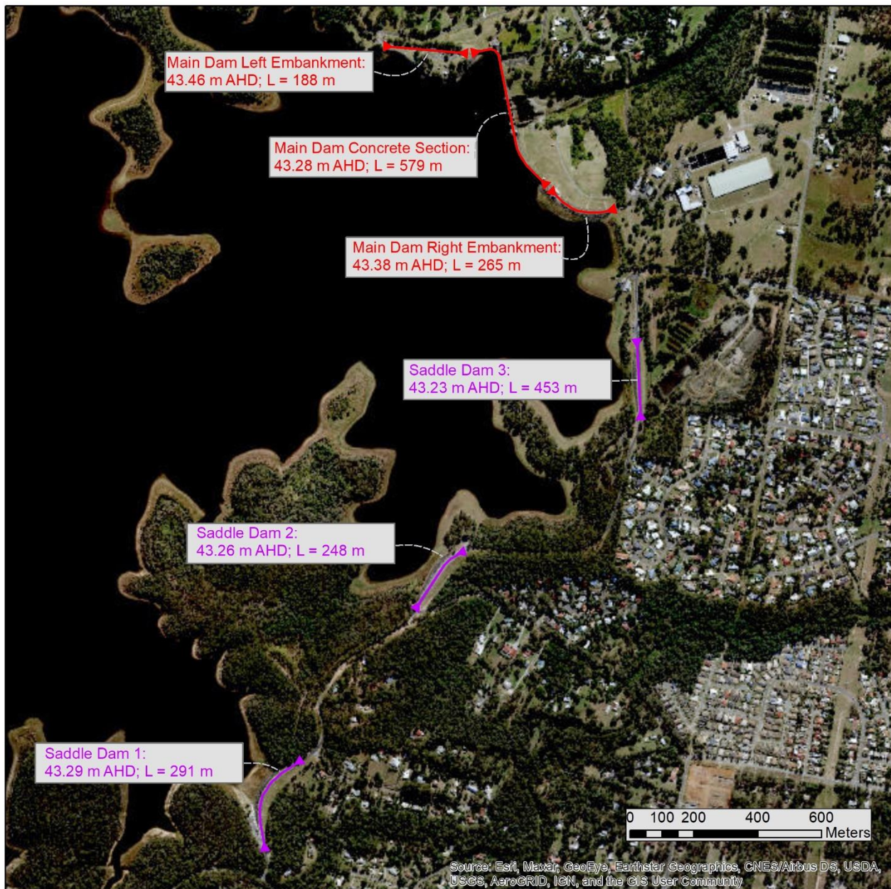
Figure 4.4.1 General layout of North Pine Dam showing component dam crest elevation and length
