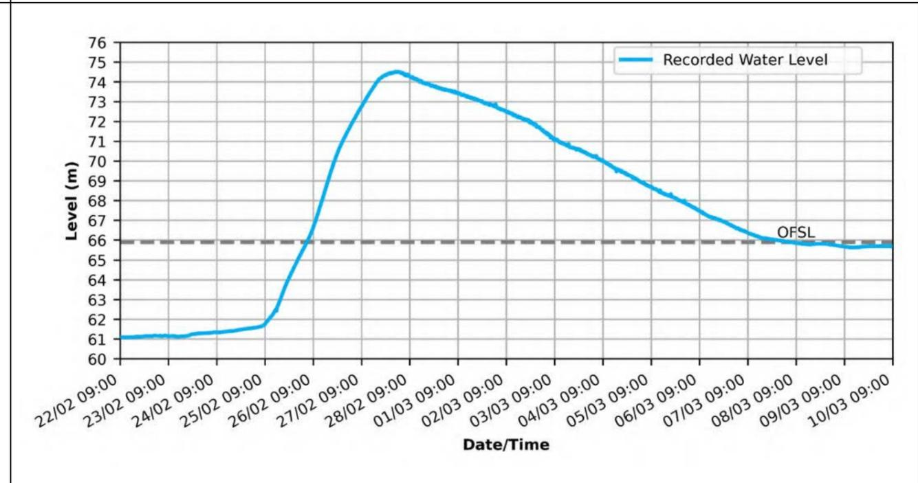
Figure 2-44: Recorded lake level at Wivenhoe Dam for the Flood Event
