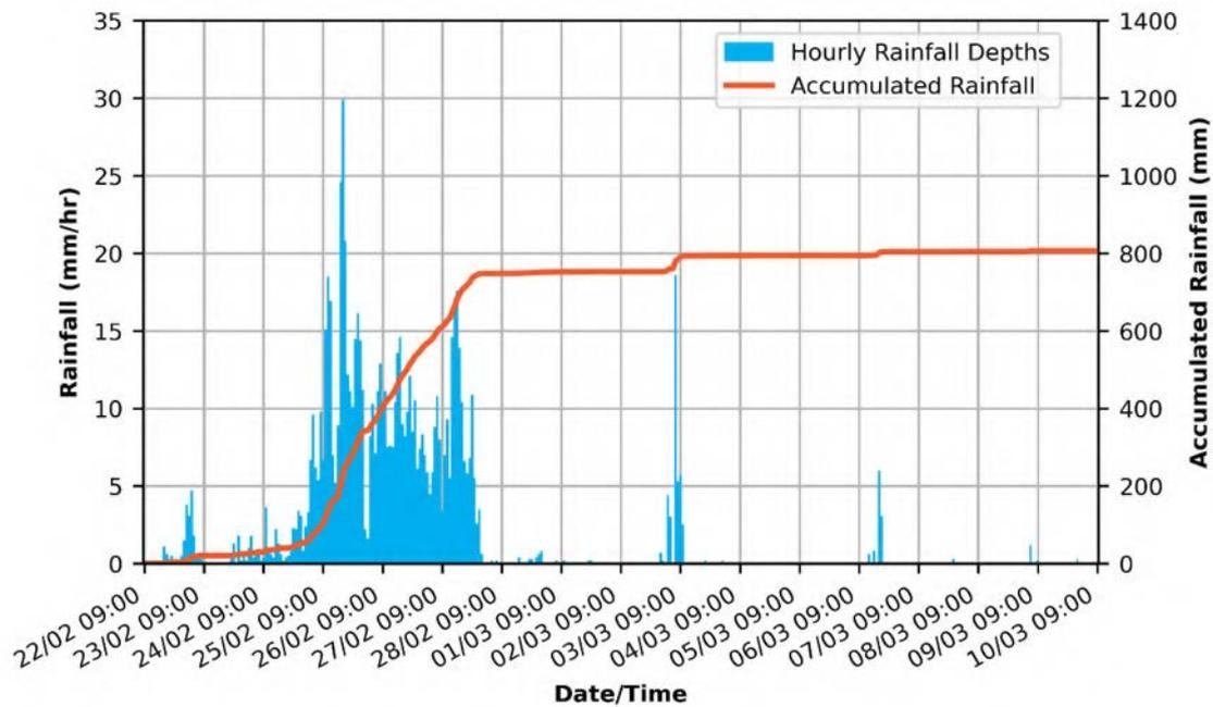
Figure 2-34: Brisbane River from Wivenhoe Dam to Moggill catchment average rainfall in hourly increments and accumulated over the Flood Event for the period 22/02/2022 09:00 to 10/03/2022 09:00
