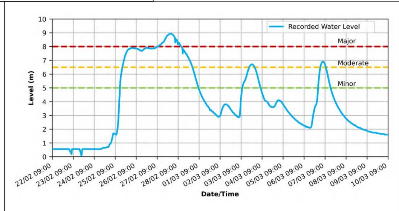
Figure 2-52: Recorded water level for Purga Creek at Loamside for the Flood Event
