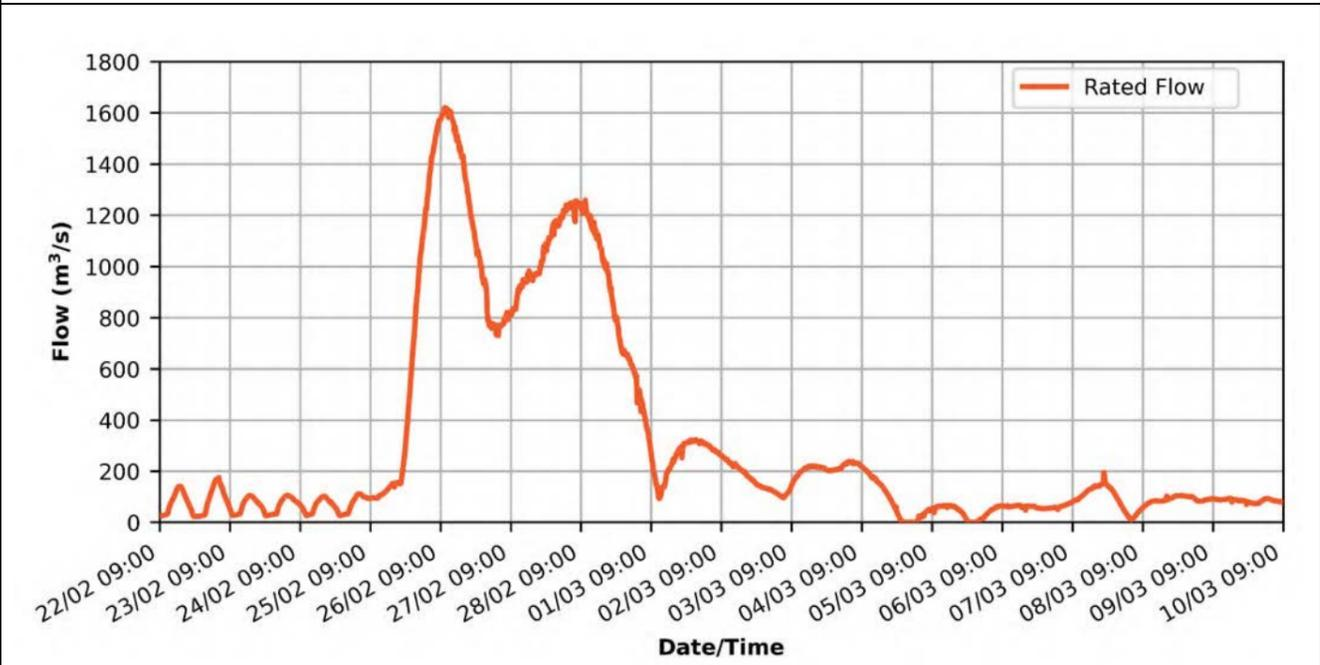
Figure 7-13: Rated flow for Bremer River at Ipswich for the Flood Event
