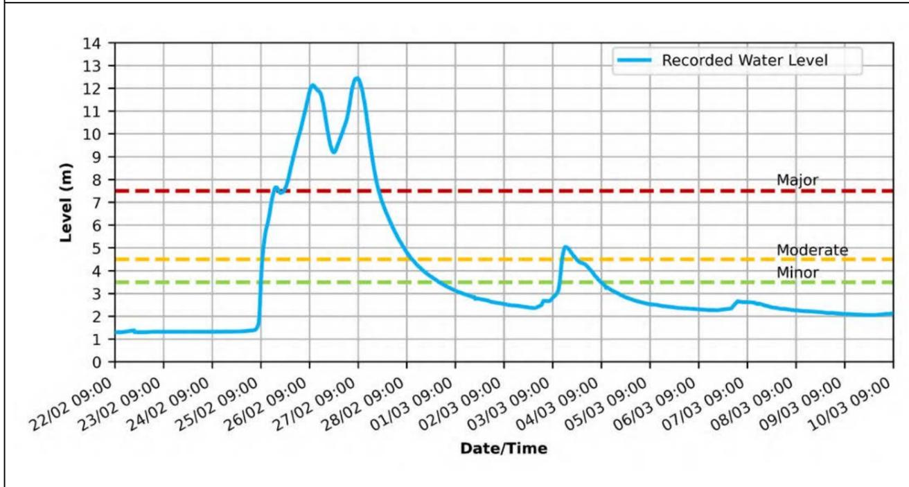
Figure 2-43: Recorded water level for Brisbane River at Gregors Creek for the Flood Event
