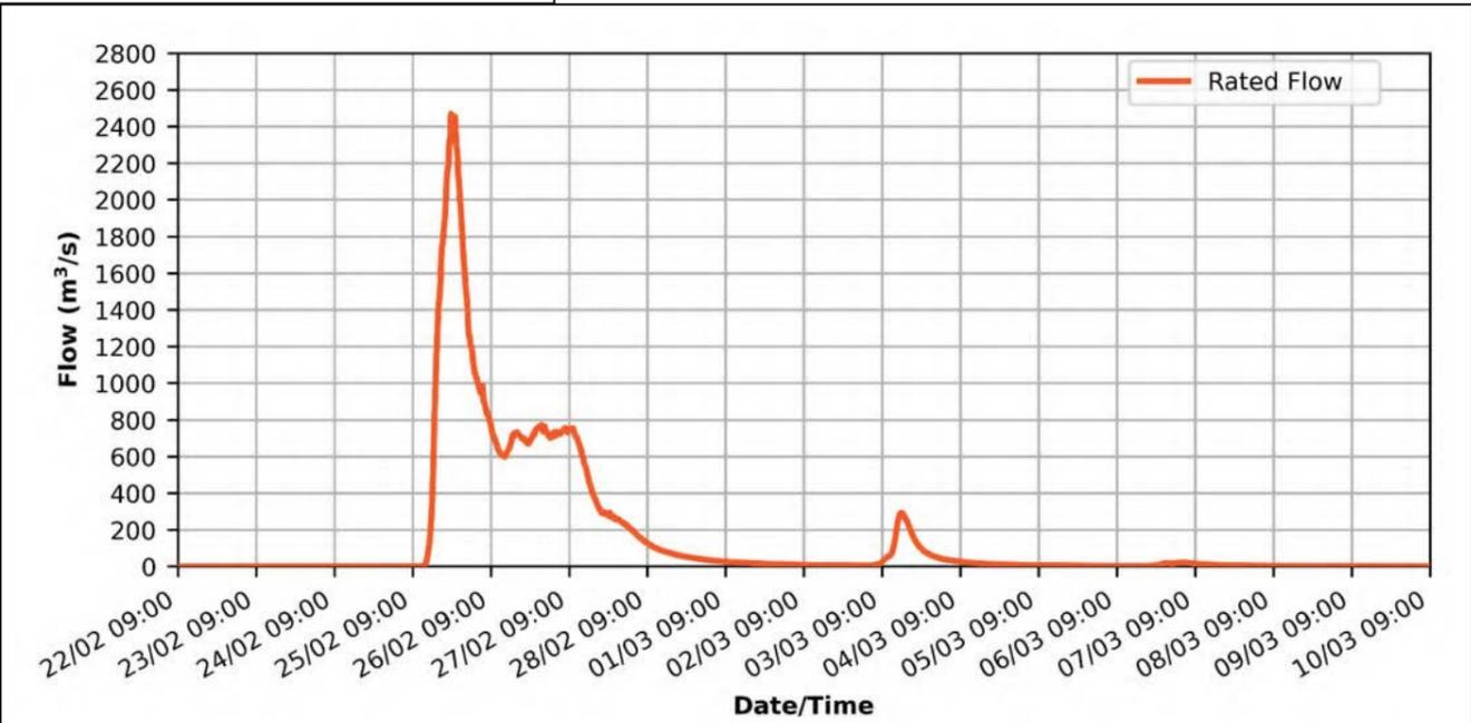
Figure 7-7: Rated flow for Lockyer Creek at Gatton for the Flood Event
