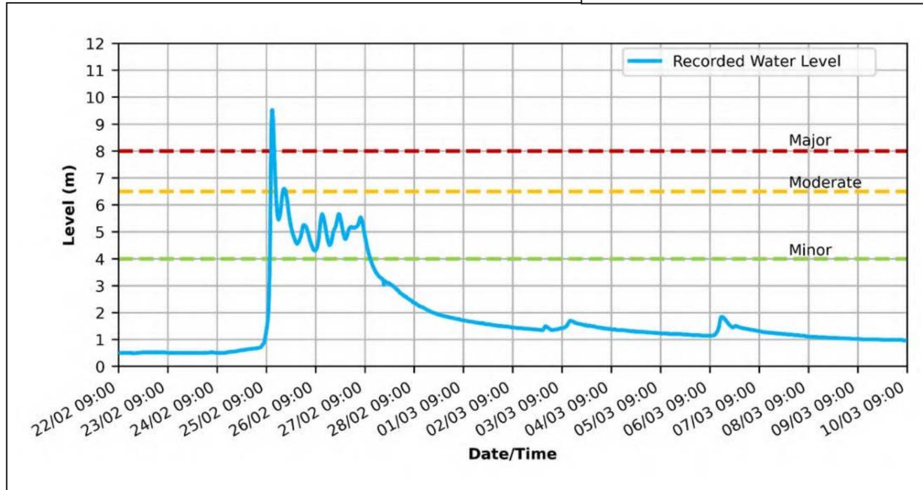
Figure 2-46: Recorded water level for Lockyer Creek at Helidon for the Flood Event
