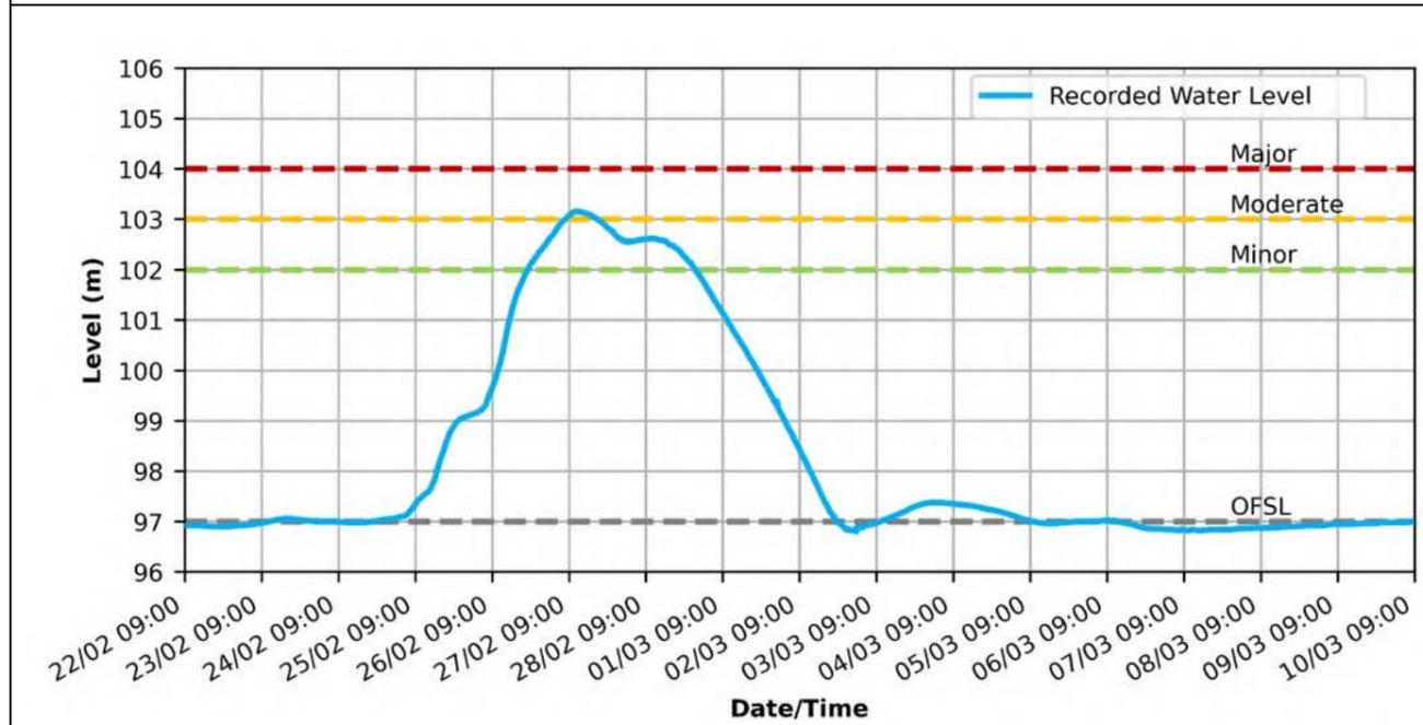
Figure 2-40: Recorded lake level at Somerset Dam for the Flood Event
