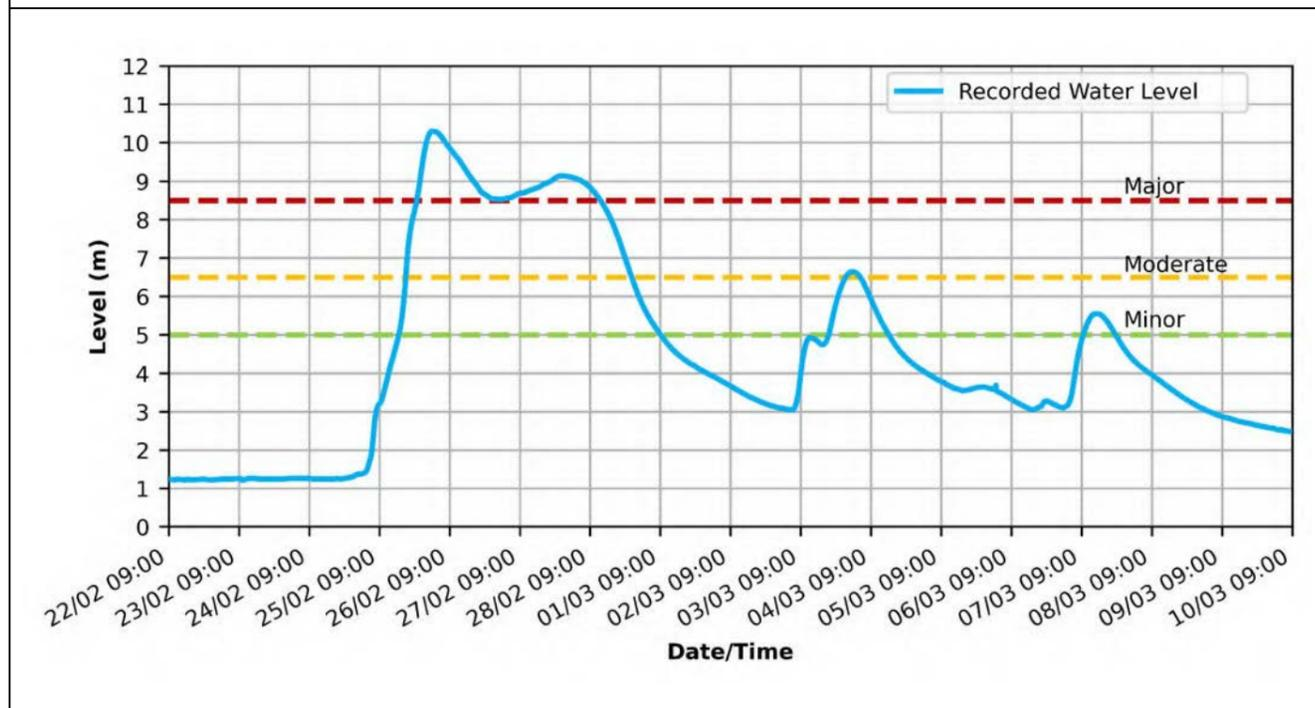
Figure 2-53: Recorded water level for Bremer River at Walloon for the Flood Event
