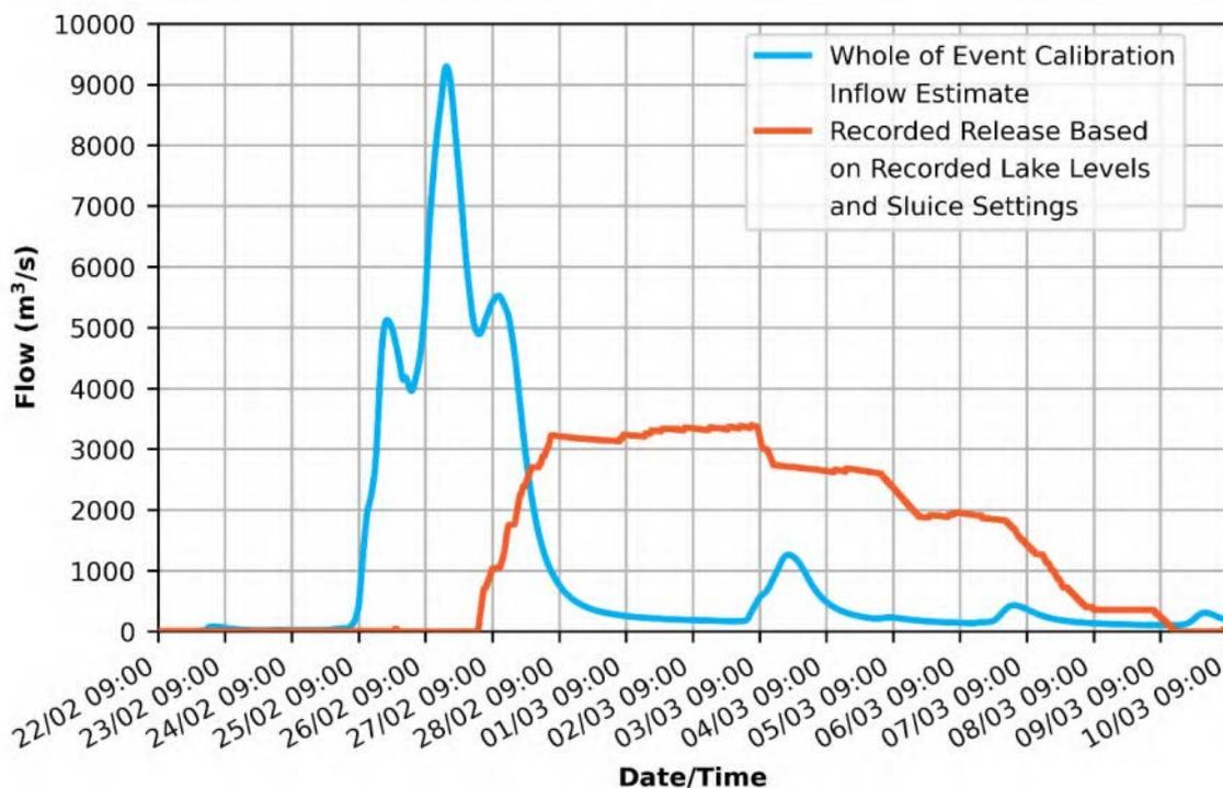
Figure viii: Wivenhoe Dam modelled inflow hydrograph produced by the post-event analysis whole of event calibration (with the benefit of hindsight) excluding Somerset Dam releases and recorded release hydrograph for the period 22/02/2022 09:00 to 10/03/2022 09:00
