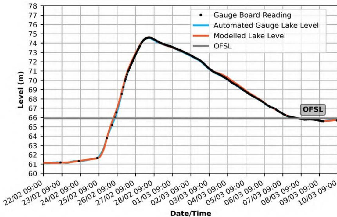
Figure vi: Wivenhoe Dam post-event analysis whole of event modelled lake level compared to automated data and gauge board readings for the period 22/02/2022 09:00 to 10/03/2022 09:00 (replicated in Figure 7-25)
