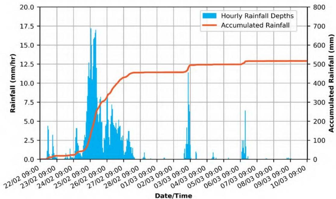
Figure 2-32: Lockyer Creek catchment average rainfall in hourly increments and accumulated over the Flood Event for the period 22/02/2022 09:00 to 10/03/2022 09:00
