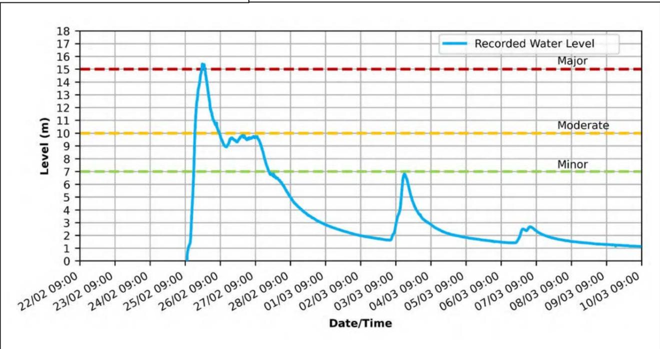
Figure 2-47: Recorded water level for Lockyer Creek at Gatton for the Flood Event
