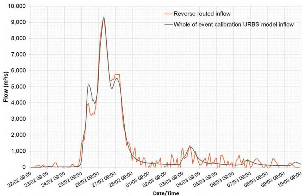
Figure 7-36: Post-event analysis reverse routed inflow calculation for Wivenhoe Dam
