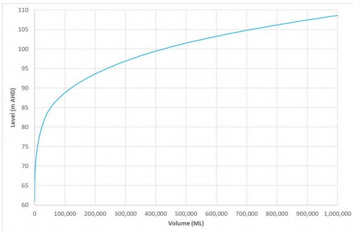
Figure 7-33: Somerset Dam storage-elevation relationship
