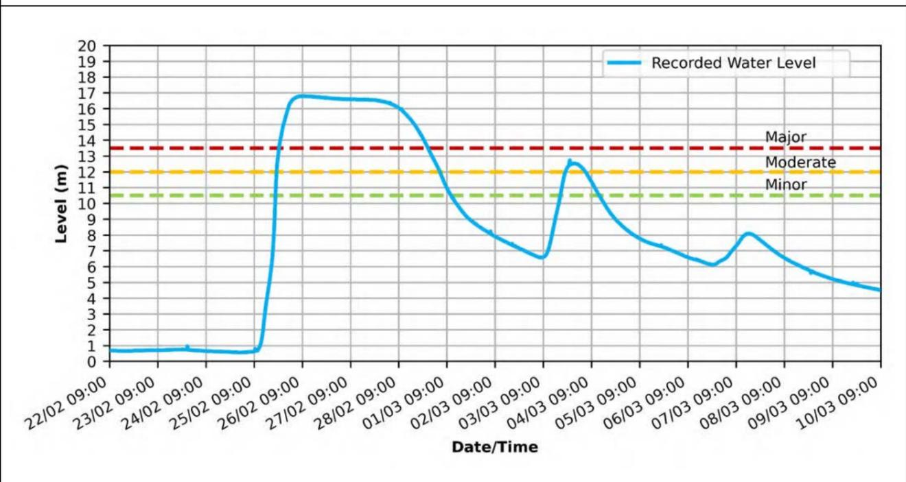
Figure 2-49: Recorded water level for Lockyer Creek at Rifle Range Rd for the Flood Event
