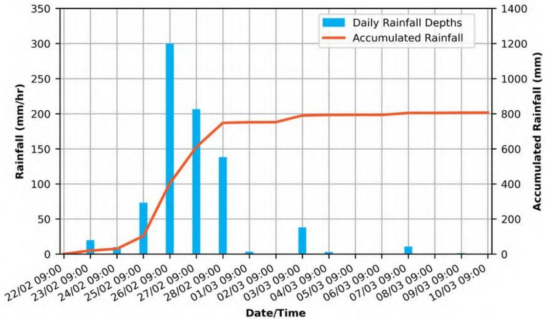
Figure 2-11: Brisbane River from Wivenhoe Dam to Moggill catchment average rainfall from 22/02/2022 09:00 to 10/03/2022 09:00
