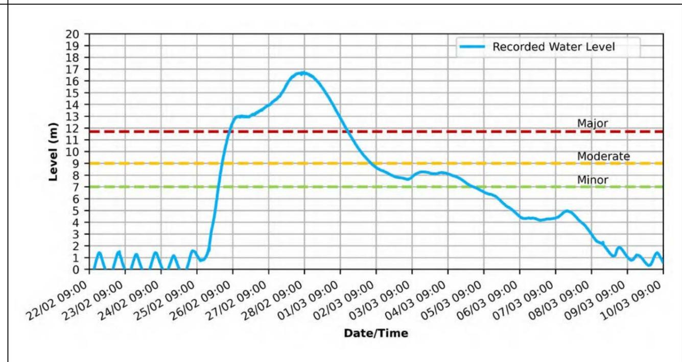
Figure 2-54: Recorded water level for Bremer River at Ipswich for the Flood Event
