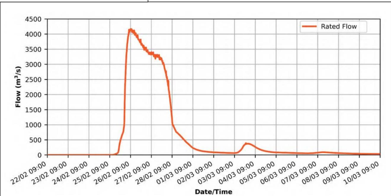
Figure 7-15: Rated flow for Brisbane River at Savages Crossing for the Flood Event
