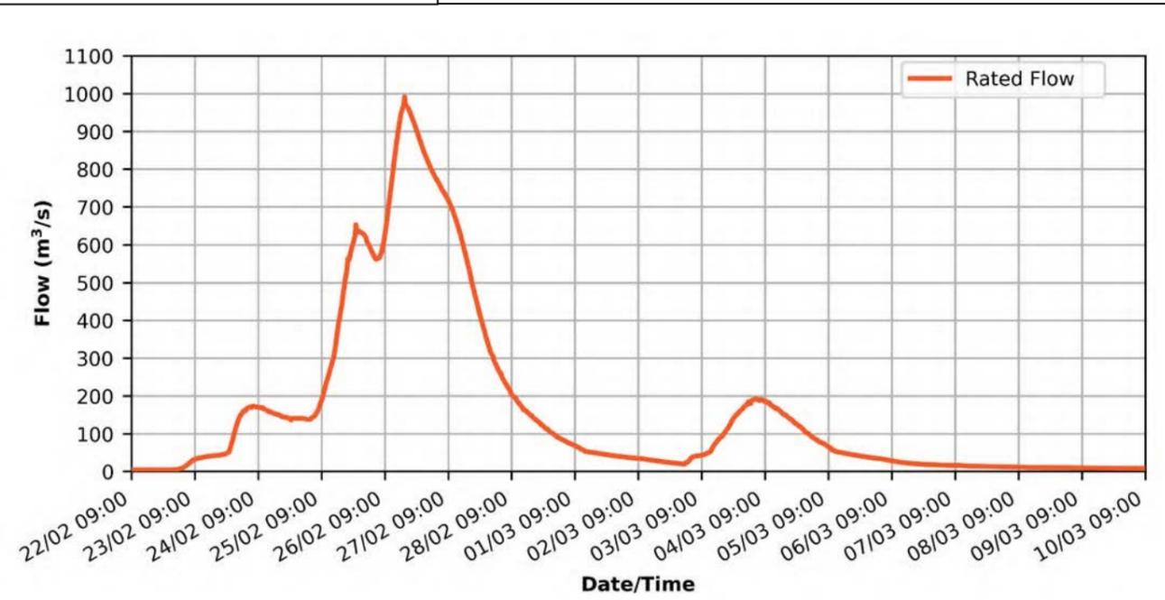
Figure 7-2: Rated flow for Stanley River at Woodford for the Flood Event
