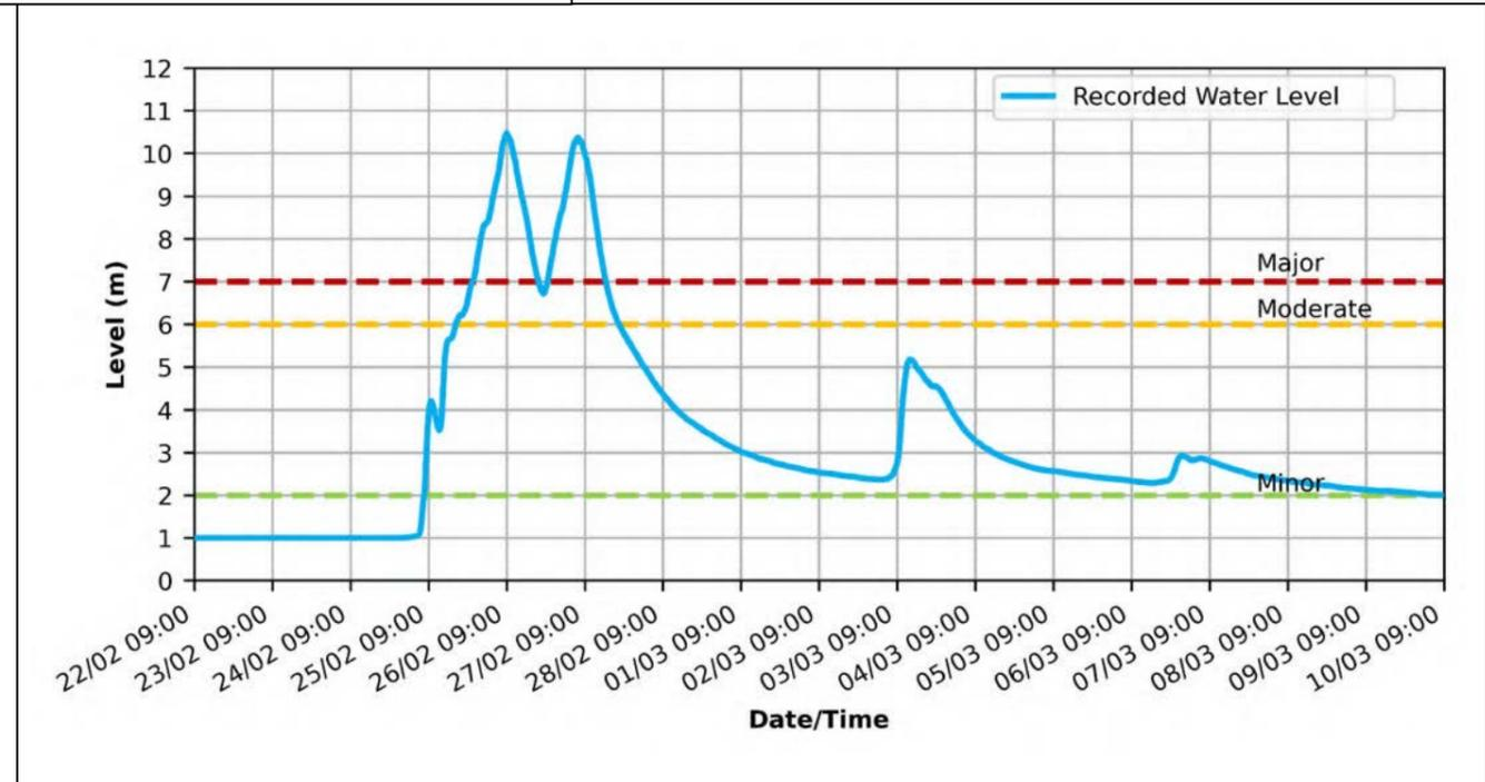
Figure 2-42: Recorded water level Brisbane River at Devon Hills for the Flood Event
