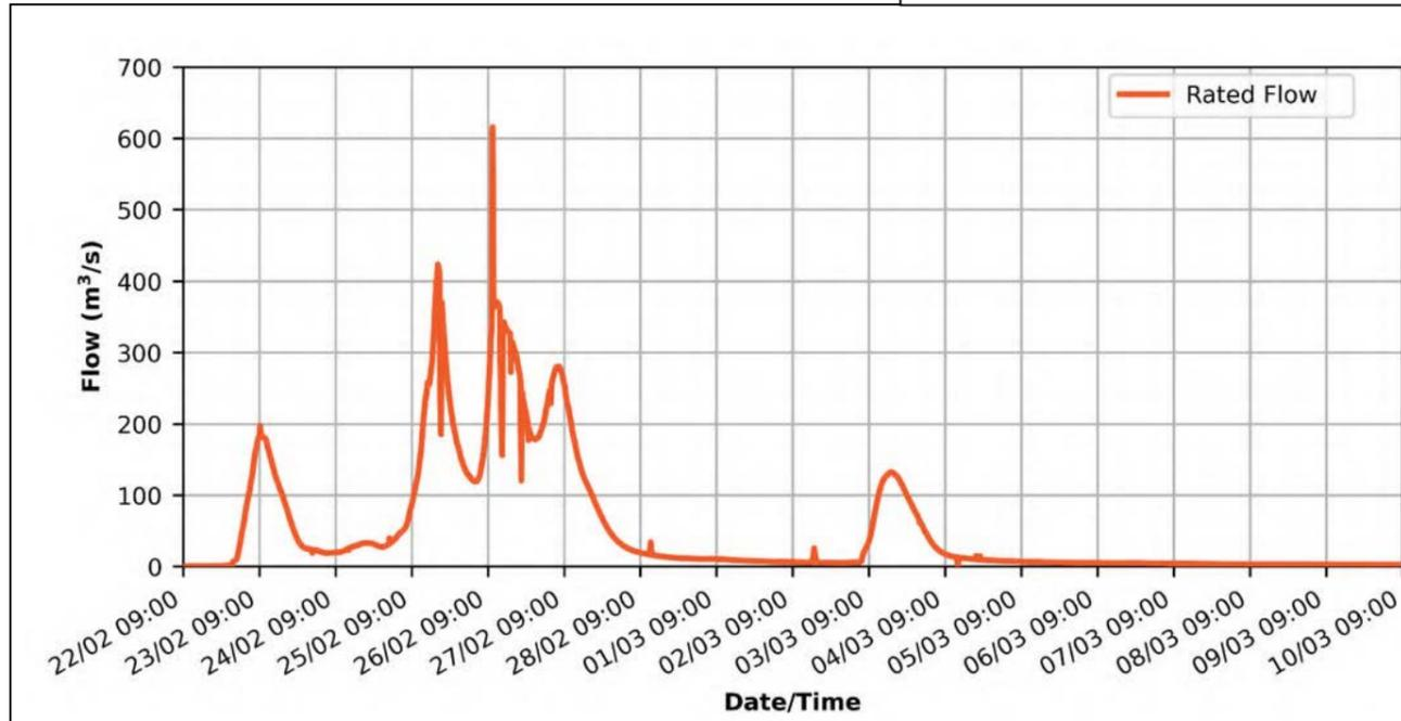
Figure 7-1: Rated flow for Stanley River at Peachester for the Flood Event
