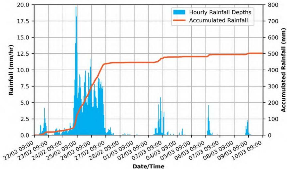
Figure iv: Brisbane River to Wivenhoe Dam catchment average rainfall in hourly increments and accumulated over the Flood Event for the period 22/02/2022 09:00 to 10/03/2022 09:00 (replicated in Figure 2-36)
