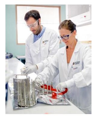
Figure 1. Preparation of a PDMS passive sampler in a stainless steel cage.
